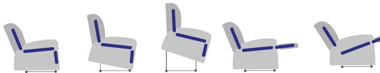
Tilt-in-space holds the user in a fixed position when in recline with the angle of the hip and the back remaining constant. This action is ideal for clients with limited torso control.
